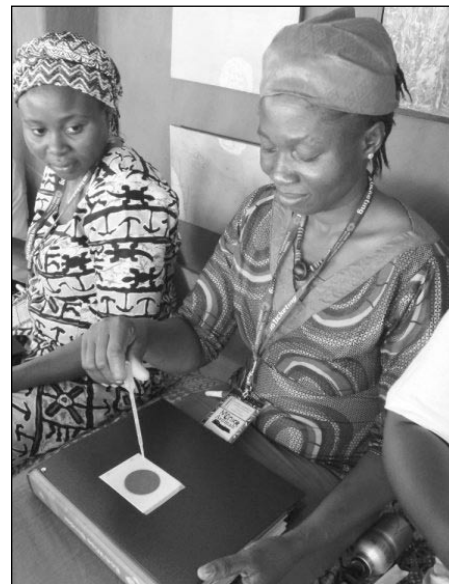
Each woman tested their home water sample by placing drops on a Petri film and incubating it overnight on their bodies.
